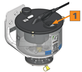
1 Pour lubricant in the top fill. Oil & NLGI #000 greases ONLY.
