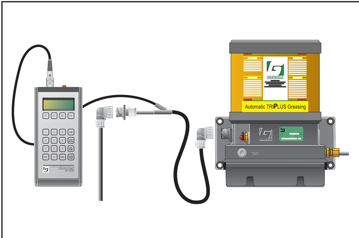
Figure 2.2 Connecting the GINA to the TriPlus pump
