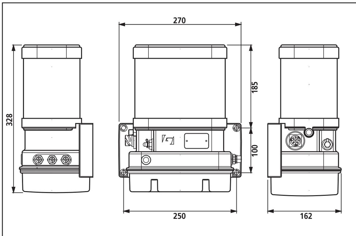
Figure 7.1 Dimensions of the TriPlus pump unit with a 3 litre reservoir.
