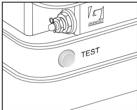
Figure 2.3 The test pushbutton
