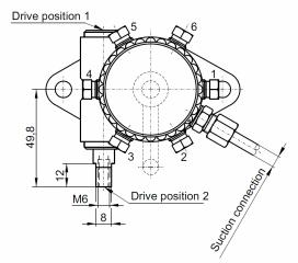
The arrangement of the pressure connections is done in the order of the numbering. If the arrangement is required in another order, this has to be indicated when the order is placed.
