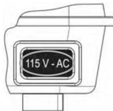
115 V - AC or 230 V - AC in the viewing window with Hirschmann plug connection Device in AC version without control unit, with Hirschmann plug connection Connection diagram see chapter 7.2.3
